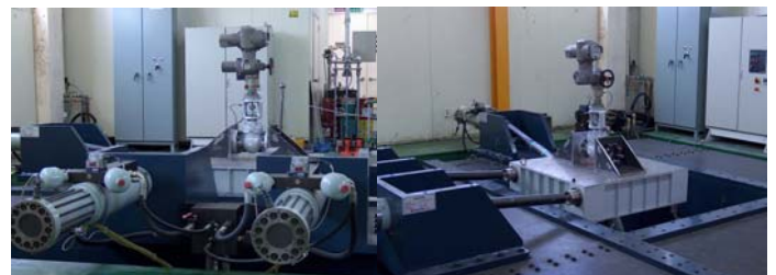
Valve on Seismic Simulator
