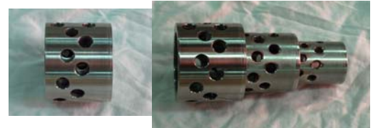
HV CAGE TRIM VALVES
